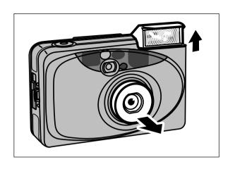
When the power is turned on, the lens cover opens, the lens unit extends toward the front and the flash unit pops up, setting the camera in a condition where it is ready to take pictures.
